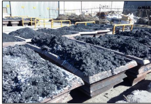
Image of Salt Slag cooling in storage containers prior to transportation for re-cycling
