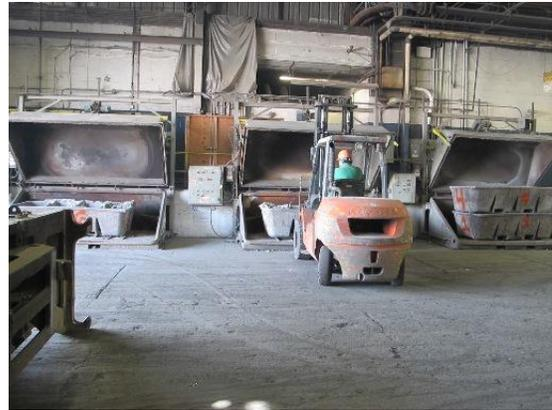
Fig. 5 Dross pan being placed in the Inert Gas Cooler
