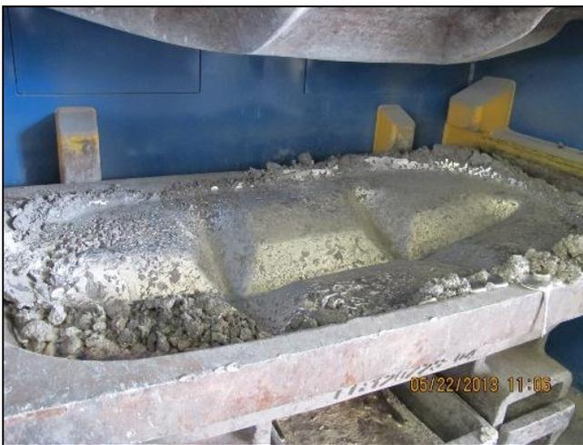
Fig. 11 Plating action generated by pressing
