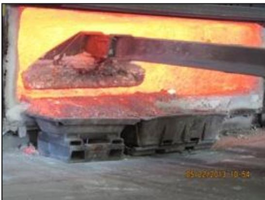
Fig. 4 Skimming into both dross pan types
