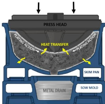
Fig. 2 Dross Press head and pan set Combination
