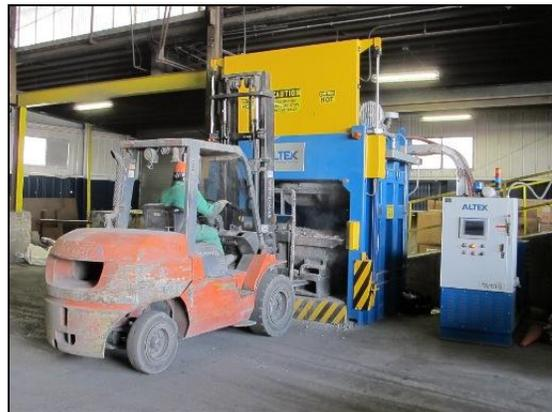
Fig. 6 Dross pan being placed in the Dross Press
