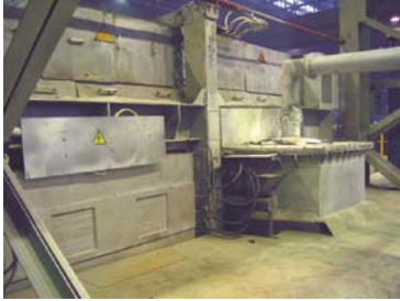
Figure 7 – Side Mounted EM ‘air cooled’ stirrer
